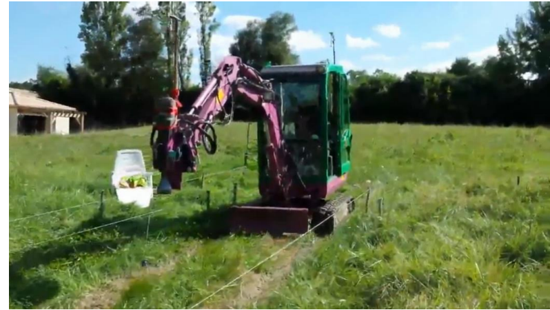
Automatic picket planting based on centimeter GPS
