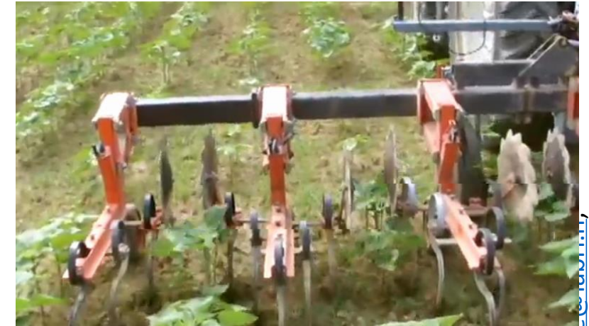
AGROGEOVISIO : Automatic weeding based on centimeter GPS coupled with vision
