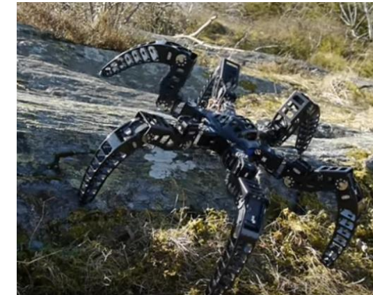
Projet HexaROV : Hexapod able to move on rough terrain (and underwater)
