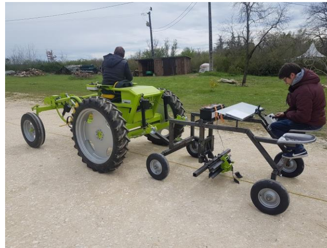
ANR BIPBIP : Intra-row weeding using a smart tool holder based on vision and control
